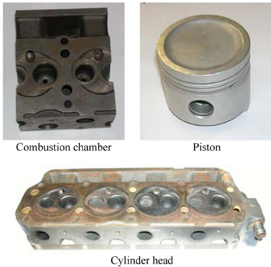
Fig. 1 Combustion chamber, piston, and cylinder head of the PAYKAN engine. Photographs have been taken using a digital camera at the Iran-Khodro Powertrain Company (IPCO).
