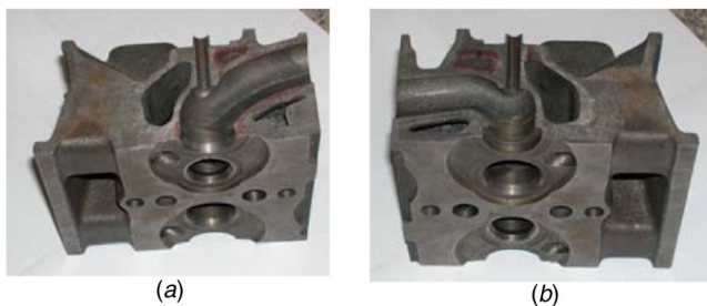
Fig. 2 A cross section of inlet port (a) and outlet port (b)
